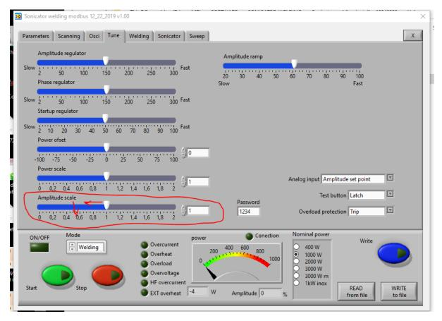
In the last software version (for 1 kW generators), we can change the measured output amplitude. See the picture. The password 1234 must be entered to be available for editing. This is instead of opening the generator and rotating potentiometers. You can adjust the output voltage, just by this software option.
